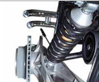
Chassis: Alloy semi-trailing link axle with adjustable Bilstein threaded suspension and 3 selectable springs: soft, medium, hard.
