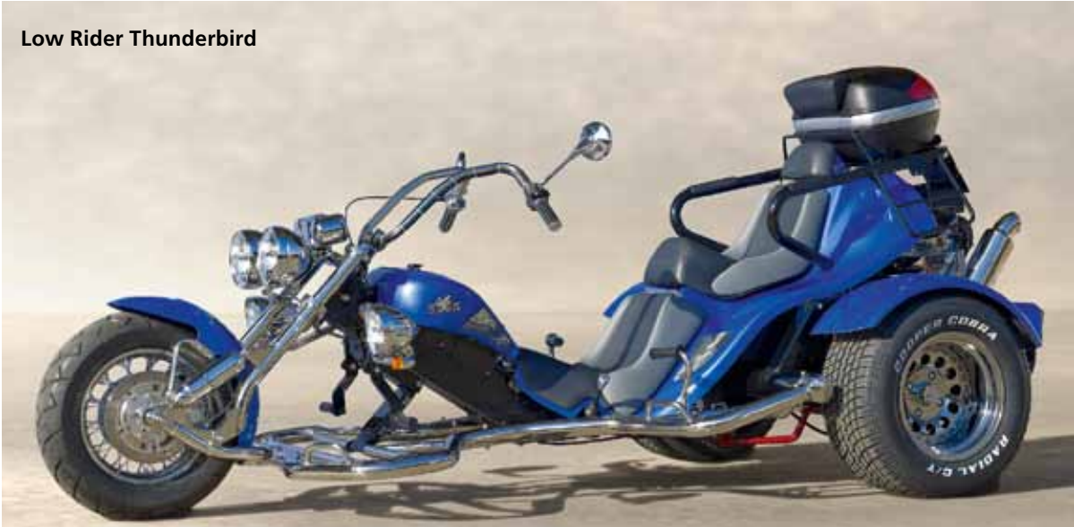
From model year 2014 without extra charge for version Thunderbird: Front wheel: 200/50-17 on 5,50x17 alloy rim, Shark Design, chrome Rear wheels: 295/50-15 on 10x15 alloy rims, Shark design, chrome
