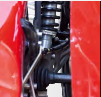
Chassis: Alloy semi-trailing link axle with adjustable Bilstein threaded suspension and 3 selectable springs: soft, medium, hard.
