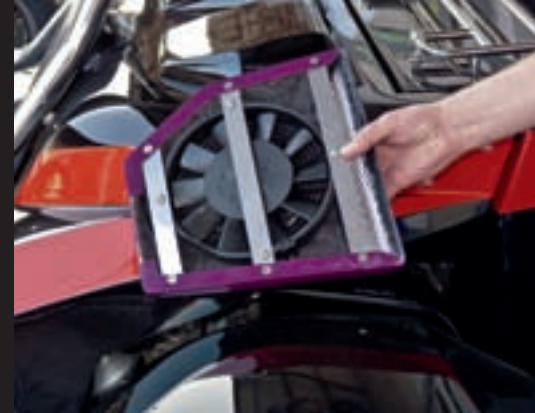
The fan in the air scoop draws hot air from the engine compartment as needed.
